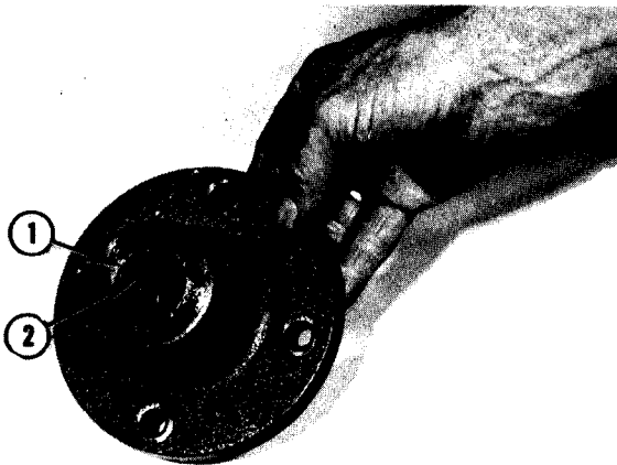
FIG. 10.7--BEARING AND SEAL INSTALLED
